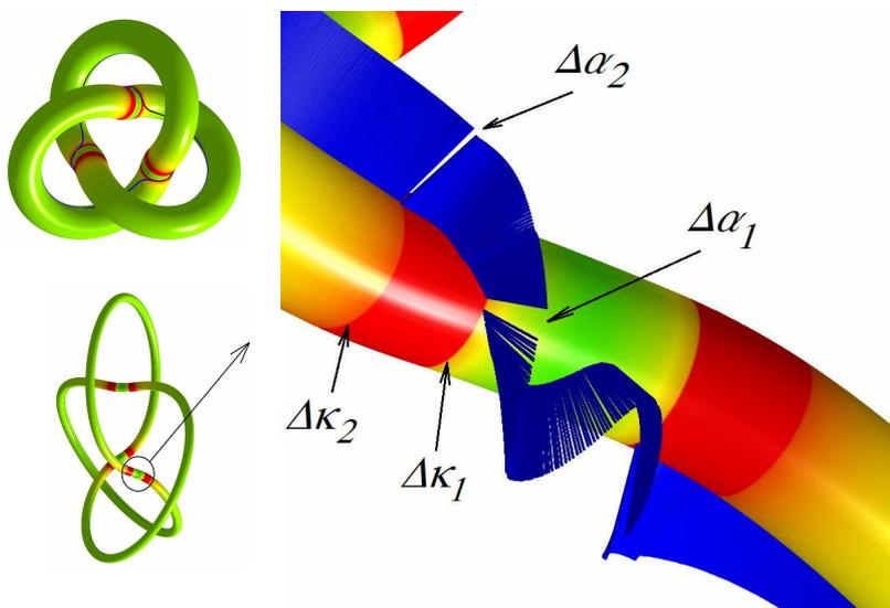
Fig. 6. The ribbon of the normal vectors in the region of the primary discontinuities.
